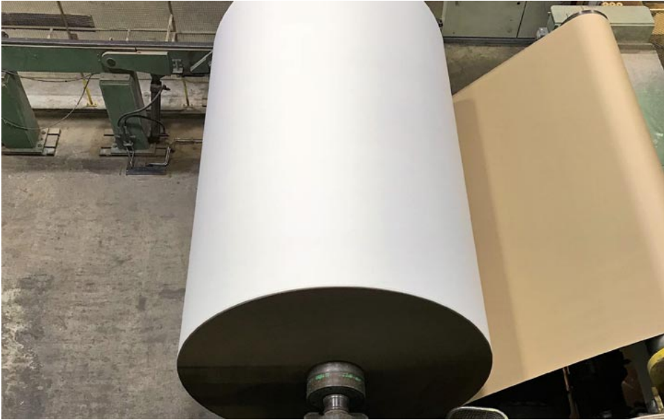
Republic Paperboard's new product, pigment coated gypsum board, produced using the new curtain coater system, which was built by Voith. (Photo: Voith)
